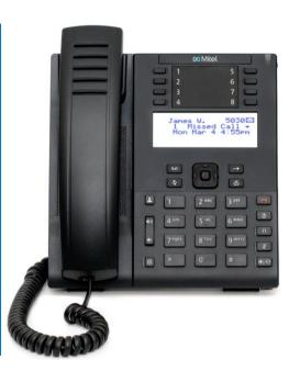
The Mitel 6910 IP Phone offers exceptional quality and standard telephony functions in an enterprise grade IP desktop phone. The Mitel 6910 features Dual Gigabit Ethernet ports and a large 3.4" LCD display with soft white backlighting and large fonts, making the screen easy to read in any lighting condition. With eight programmable keys, native DHSG/ EHS analog headset support, and high definition audio quality, the Mitel 6910 IP Phone is ideal for business of all sizes.
